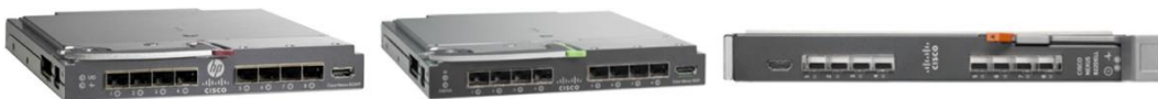
Figure 10. From Left to Right: Cisco Nexus B22HP Fabric Extender, Cisco Nexus B22F Fabric Extender, Cisco Nexus B22DELL Fabric Extender
